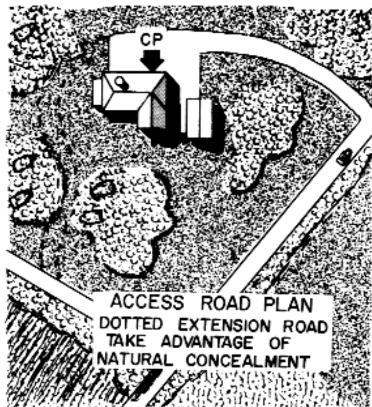
Figure 49. By continuing existing road (dotted lines) a traffic loop is created. This makes a conspicuous turn around unnecessary. It also provides access to vehicle park concealed in woods at a distance from the CP.
