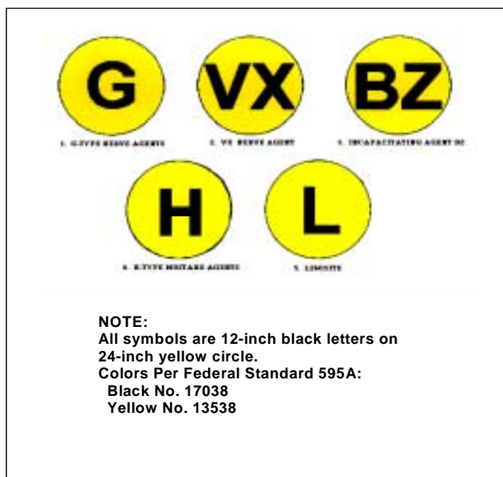
Figure 8-5. Supplemental Chemical Hazard Symbols
