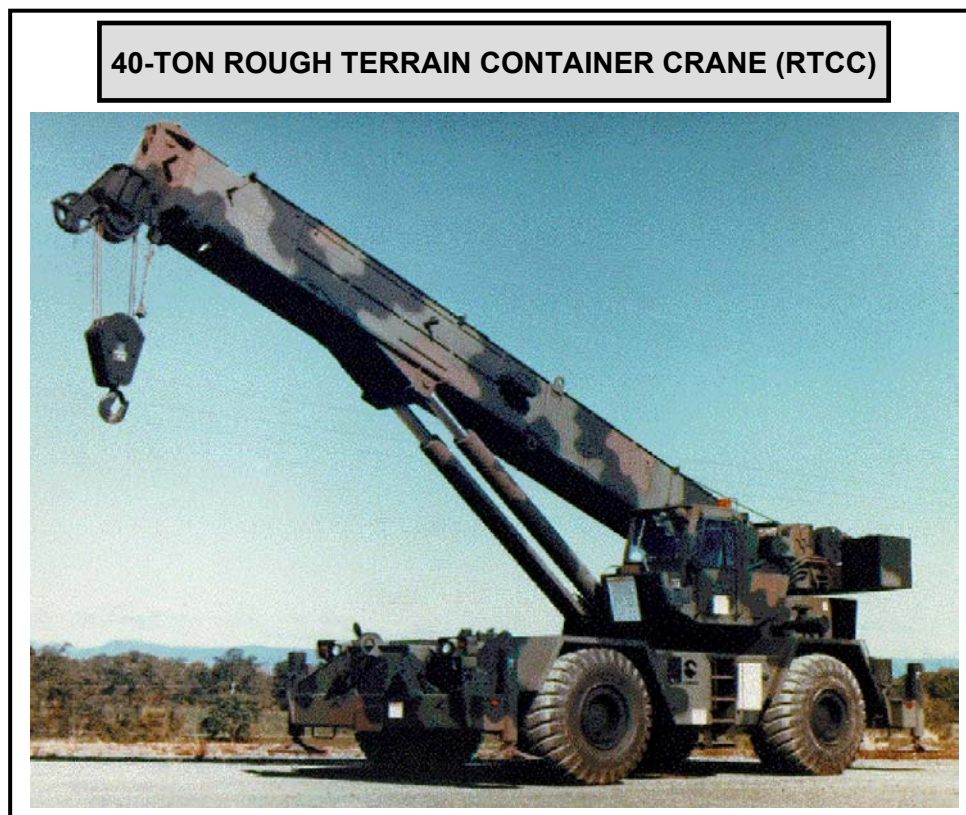
Figure J-3. 40-Ton Rough Terrain Container Crane
