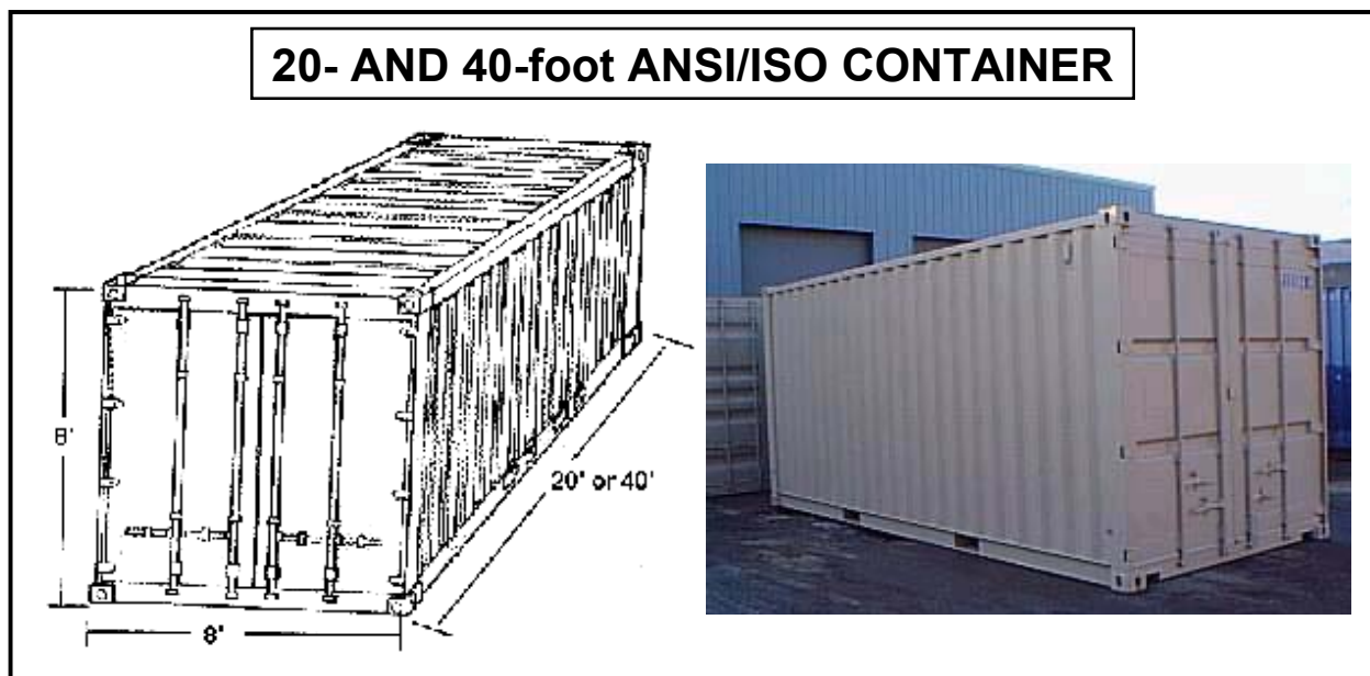
Figure J-9. Common Intermodal Container
