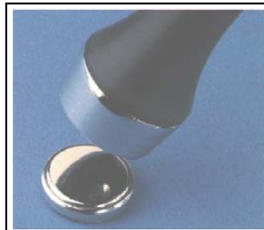
Figure C-7. Contact Memory Button and Probe
