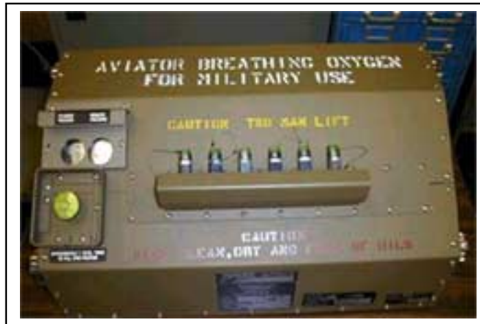
Figure 10-1. Helicopter Oxygen System
