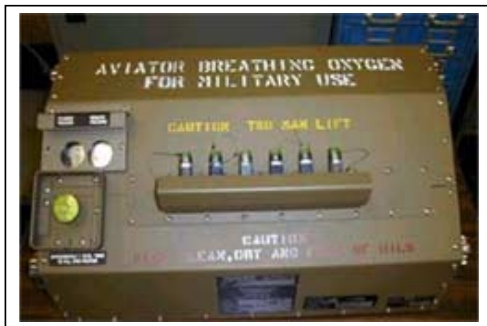
Figure 10-1. Helicopter Oxygen System
