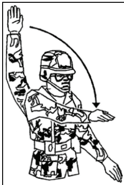
Figure A-24. Tail to right (starboard) Point left arm down, and move right arm from overhead vertical position to horizontal forward position. Repeat right arm movement.
