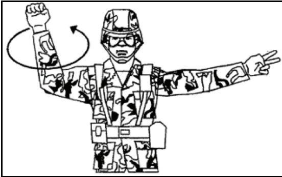
Figure A-18. Start engine(s) Day. Left hand overhead with appropriate number of fingers extended to indicate the number of the engine to be started and circular motion of right hand at head level. Night. Similar to day signal except that the wand in the left hand will be flashed indicating the engine to be started.
