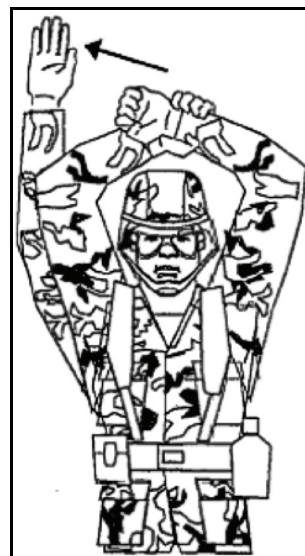
Figure A-44. Remove Day. With arms and hands in "install-downlocks" position, the right hand unclasp the left forearm. Night. Similar to the day signal except that the right wand is placed against the left forearm. (Downlocks/Undercarriage Pins)
