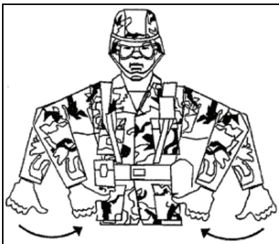
Figure A-34. Insert chocks/chocks inserted Arms down, fists closed, and thumbs extended inward. Swing arms from extended position inward.
