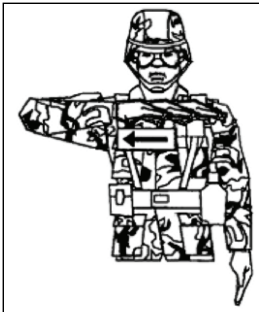
Figure A-31. Cut engine(s) or stop rotor(s)
