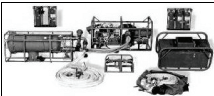
Figure 3-9. Forward area refueling equipment kit assembly
