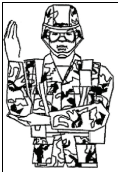
Figure A-42. Lock wings/helicopter blades Hit right elbow with palm of left hand
