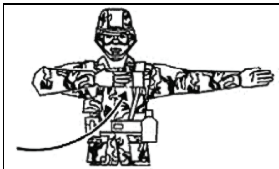
Figure A-2. Proceed to next ground guide Both arms extended on same side of shoulder level to indicate direction of next ground guide.
