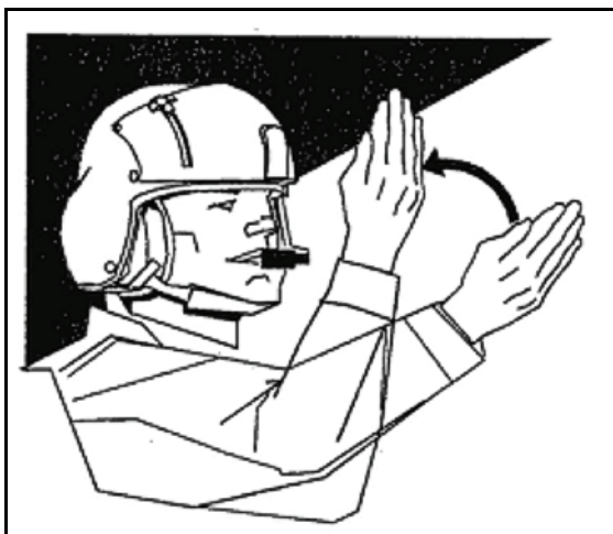
Figure A-26. Clearance for personnel to approach aircraft A beckoning motion with right hand at eye level.
