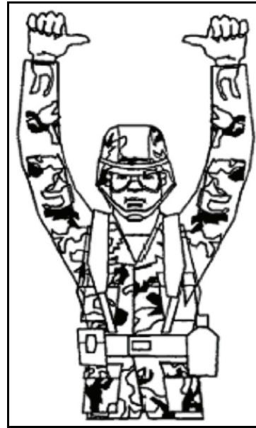
Figure A-47. Droop stops in When droop stops go in, ground guide turns thumbs inward.
