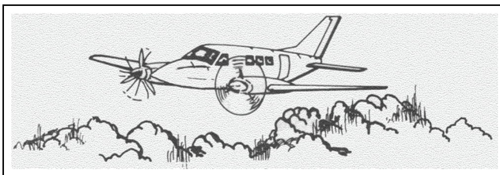
Figure 7-62. Windmilling propeller creating drag
