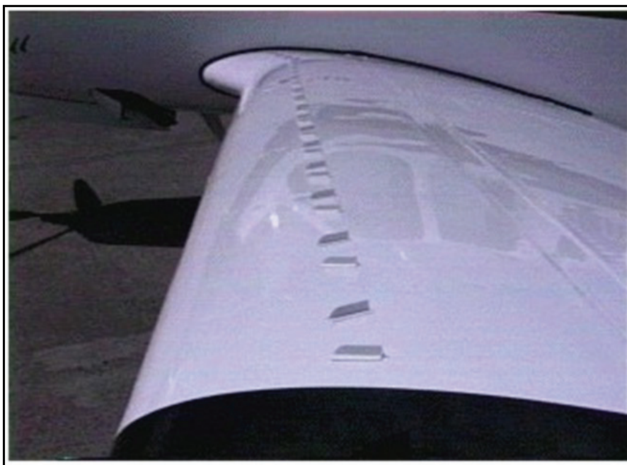
Figure 7-26. Vortex generators
