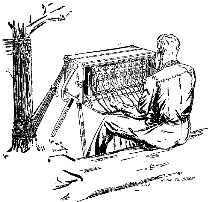
FIGURE 117.—Switchboard BD-72 set up for operation.
