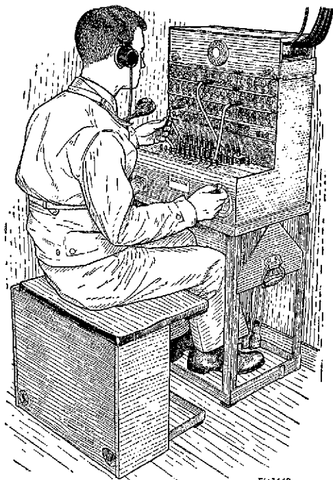
FIGURE 124.—Switchboard BD-96 set up for operation.
