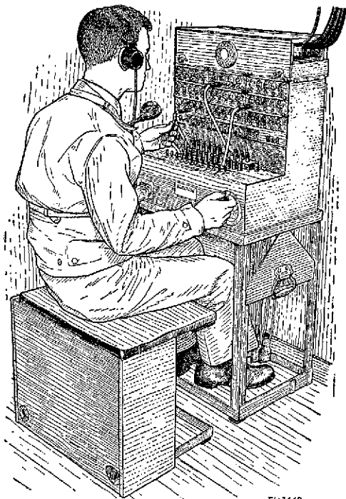
FIGURE 124.—Switchboard BD-96 set up for operation.
