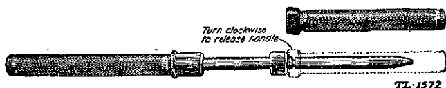
FIGURE 108.—Axle RL-27 showing removable handle.
