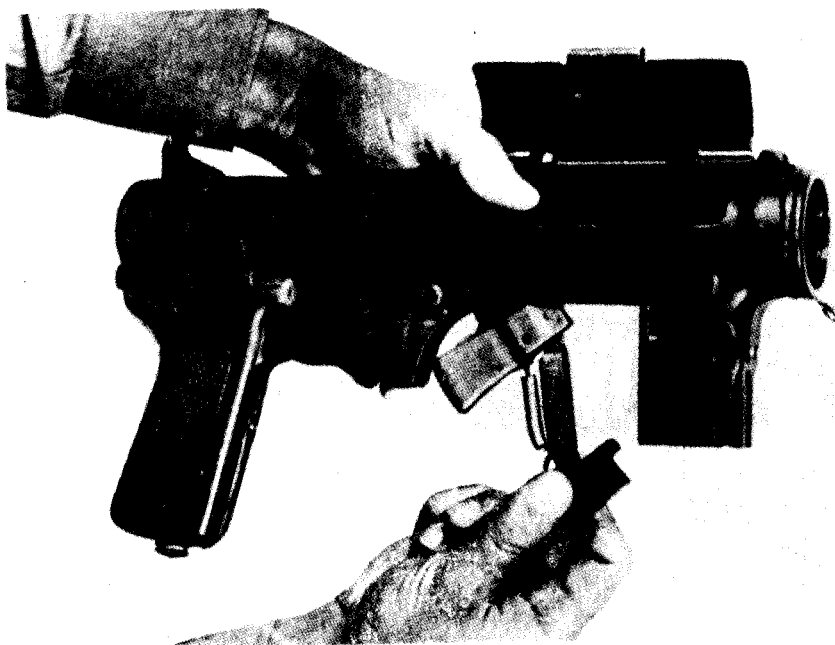
Figure 14. Withdraw the trigger and sear group from the receiver. Be careful not to drop the connector pin. This completes field disassembly.
