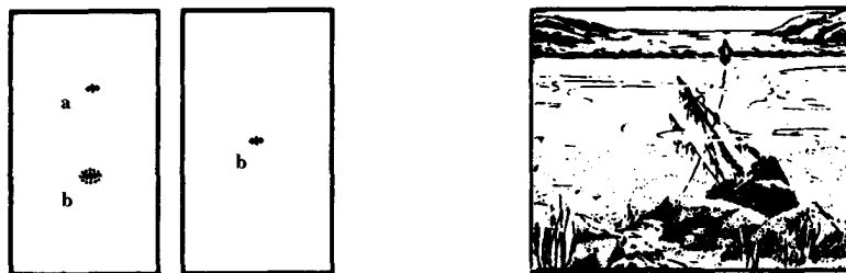
Figure 89. Sunken Danger or Obstruction. Labeling indicates the nature of the feature.
