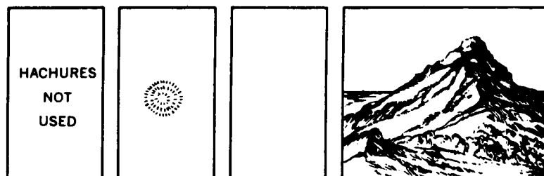
Figure 43. Hachures. This symbol is used to indicate significant formations not revealed by contours.
