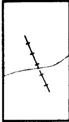
Figure 205. Tank. Tanks which are used for storage of oil, gas, water, vinegar, or other liquids. Labeling usually describes the contents. Large tanks are plotted to scale on large-scale maps.
