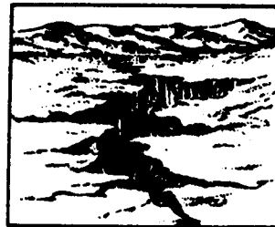
Figure 49. Cut. Cuts less in depth than the contour interval are usually omitted.
