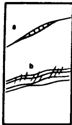
Figure 49. Cut. Cuts less in depth than the contour interval are usually omitted.
