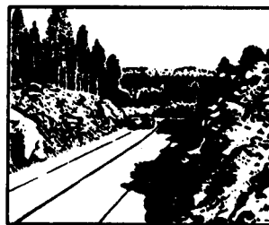
Figure 50. Fill. Fills less in height than the contour interval are usually omitted, except in extremely flat areas.
