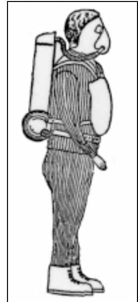
Figure 1-9. Fleuss Apparatus.
