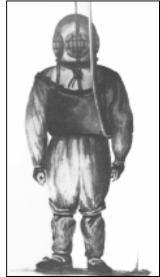
Figure 1-5. Siebe's First Enclosed Diving Dress and Helmet.
