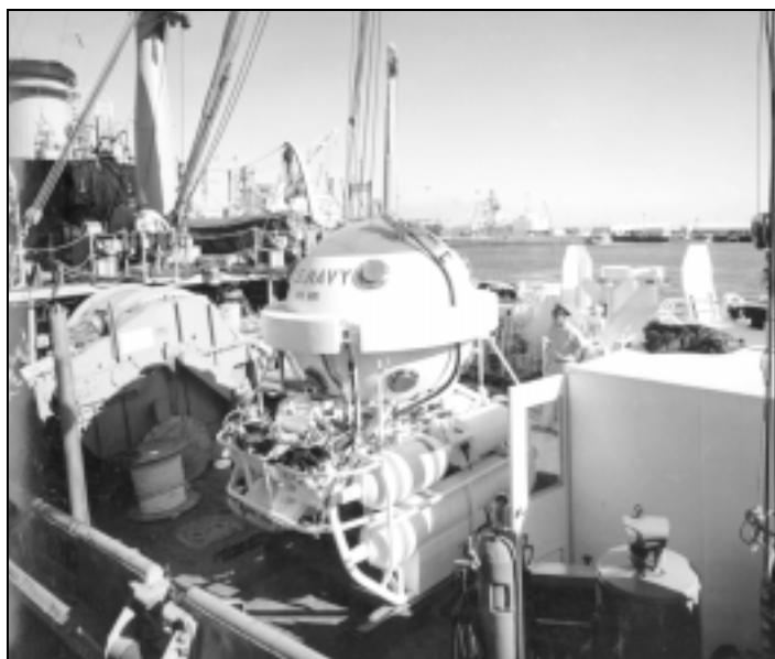
Figure 1-19. DDS MK 1 Personnel Transfer Capsule.
