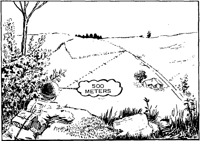
Figure 120. (Superseded) Applying the 100-meter unit of measure for ranges up to 500 meters.
