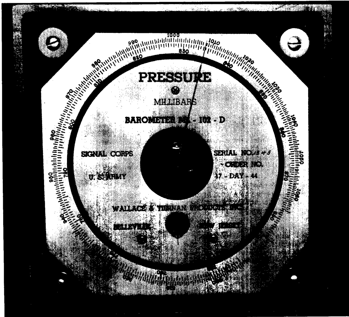
Figure 5-2. Aneroid barometer.
