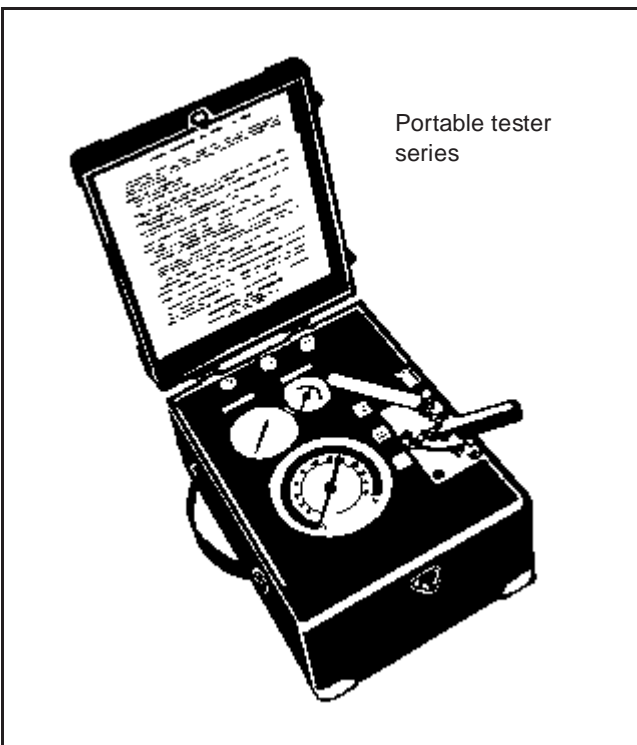
Figure 2-20. Portable hydraulic-circuit tester
