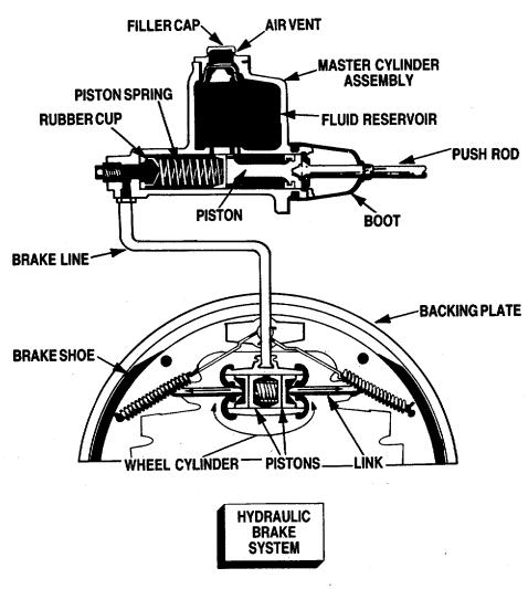
b. When brake shoes press hard against a drum or rotor, they develop friction. This friction does-the braking. The truck stops as long as you have good brake linings and an airtight hydraulic system filled with fluid.
