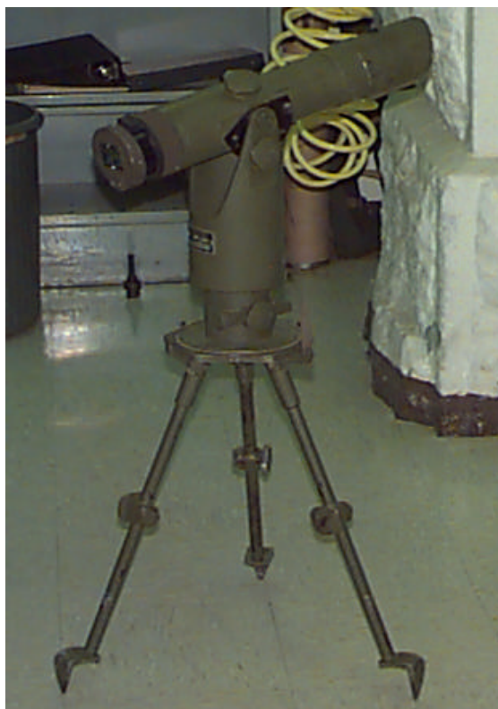
Figure 3-A: M1A1 Infinity Collimator (contains 10 Ci of Tritium)
