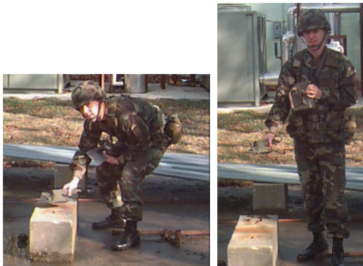
Figure 7-F: The X-Ray probe and the control unit is shown on the left. The proper use of the probe is shown on the right.
