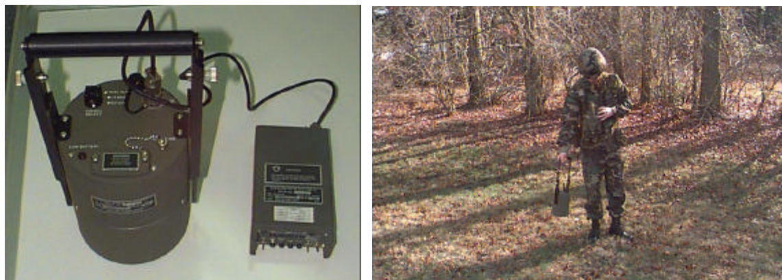
Figure 7-F: The X-Ray probe and the control unit is shown on the left. The proper use of the probe is shown on the right.
