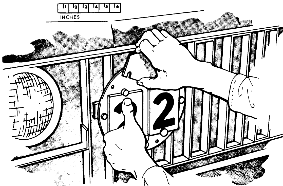
Figure 2-8. Unlocking the retaining plate.
