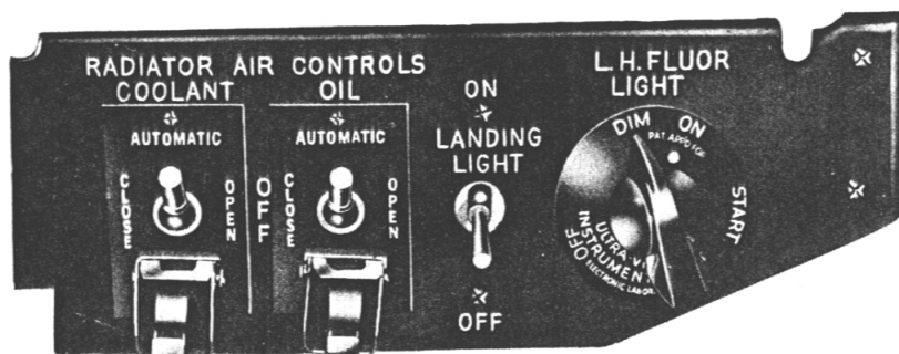
Figure 19—Radiator Air Control Panel
