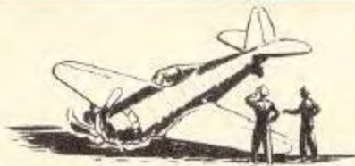
NOSING UP BY SLAMMING ON BRAKES
