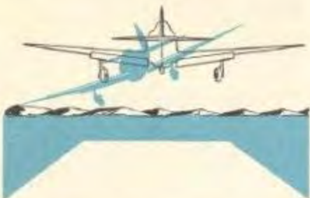
WHEN GOING AROUND—APPLY POWER SMOOTHLY TO AVOID EXCESSIVE TORQUE
