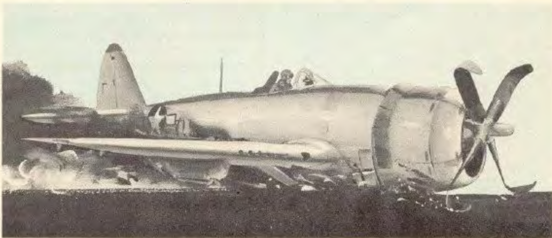
DROP EXTERNAL TANKS BEFORE MAKING A BELLY LANDING. THEY CATCH FIRE.
