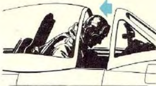
WHEN RELEASING CANOPY IN FLIGHT - DUCK
