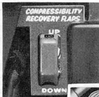
Figure 16— Compressibility Recovery Flap Switch
