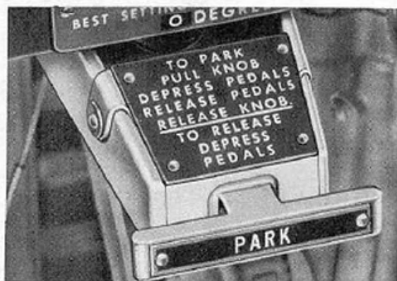
Figure 24—Parking Brake Control Through P-47D-28
