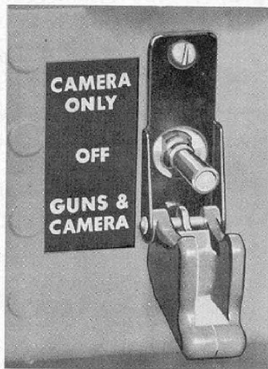
Figure 47—Gun Safety Switch
