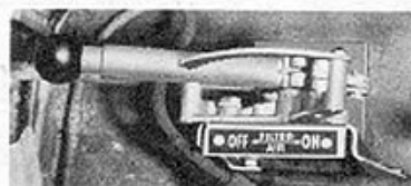
Figure 14— Air Filter Control
