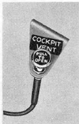
Figure 20— Cockpit Vent Control
