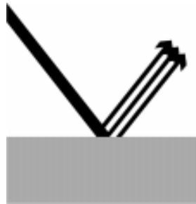
Fig.14 Semi-specular reflection
