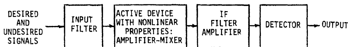
Figure 3-48. Block Diagram of Basic Receiver Elements
