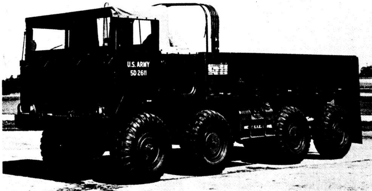
Figure 1-7. Cargo Truck, 5-ton, 8 X 8, M656
