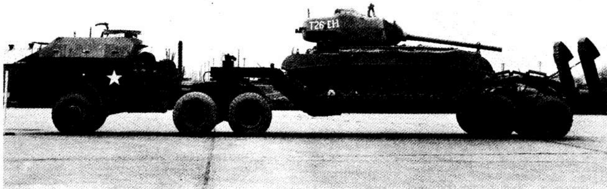
Figure 1-14. Truck Tractor, 12-ton, 6 X 6, M26A1 With Tank Transporter Semitrailer, 50-ton, 8-wheel, M15A2
