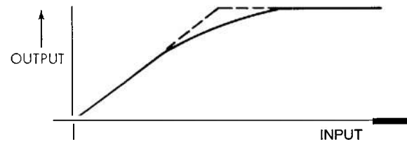
Figure 2-15. Plot depicting the limiting type of nonlinearity.
