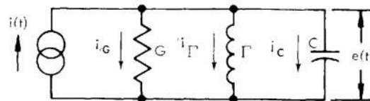
(B) Parallel RLC circuit in which current is analogous to force in (A).
