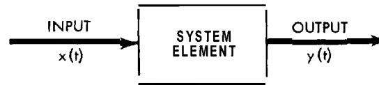
Figure 4-29. Functional representation of a system element with a single time-varying input and a single time-varying output.
