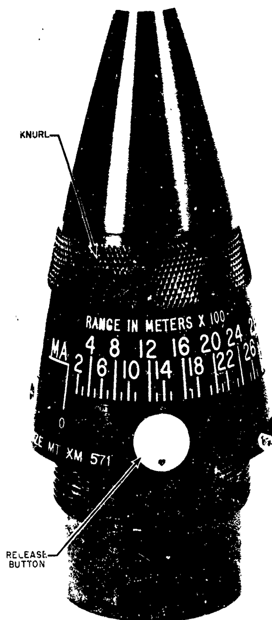
Figure 2-3. Setting Mechanism on Fuze, MT, XM571
