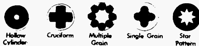
Fig. 2-6 Geometry of some rocket solid propellant charges.
