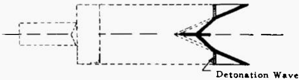
(b) Hollow charge undergoing process of a high explosion. The detonation wave initiated by the detonator and booster has passed over most of the liner which is in the process of collapsing to form the jet and slug. At this stage, the principal liner mass in the jet has been formed from the apex of the liner.
