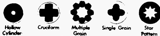
Fig. 2-6 Geometry of some rocket solid propellant charges.
