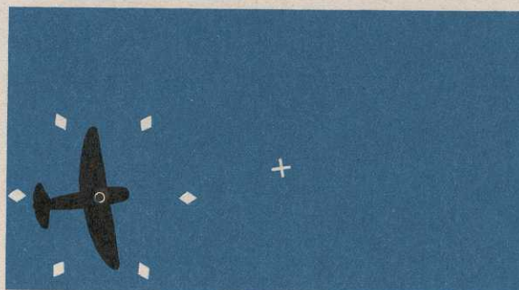
Incorrect—Imaginary circle formed by inner tips of diamonds should correspond to target's wing span.
