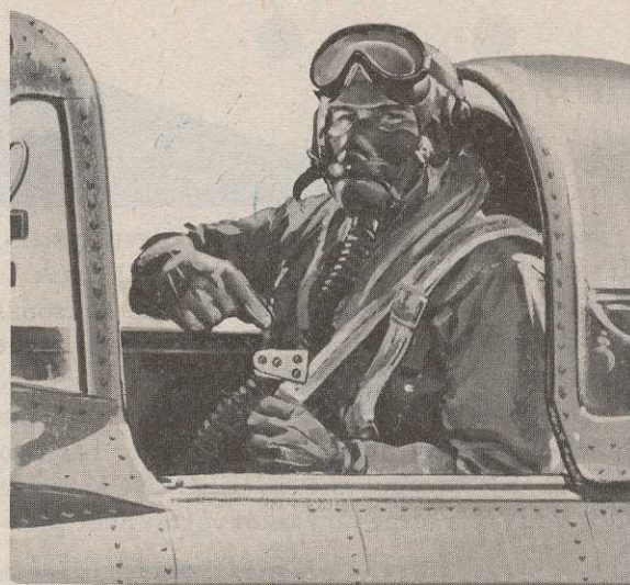
Clip oxygen hose to shoulder harness, not parachute harness, to afford quick getaway
