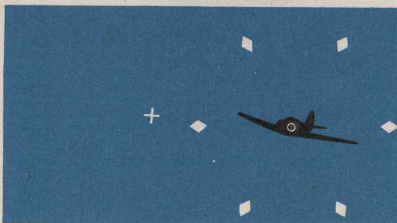
Incorrect—Circle of diamonds is too large, making range and lead angle wrong.
