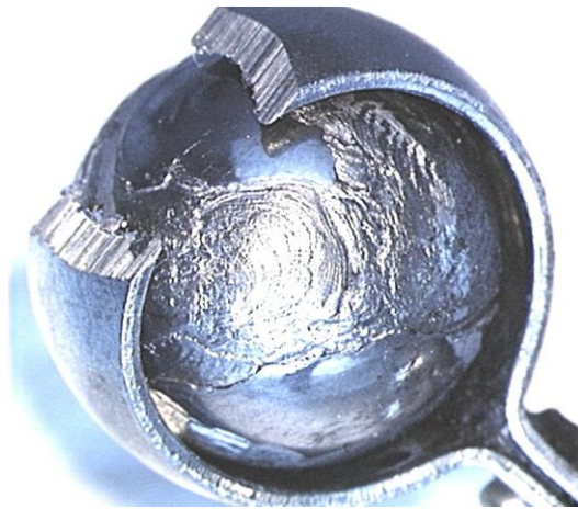
FIGURE D-12. Damaged ball from 01-05270 aft hanger bearing
