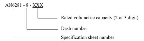
Example: AN6281-8-20 indicates fuse, 0.5 inch OD tubing with rated capacity of 20 cubic inches.
