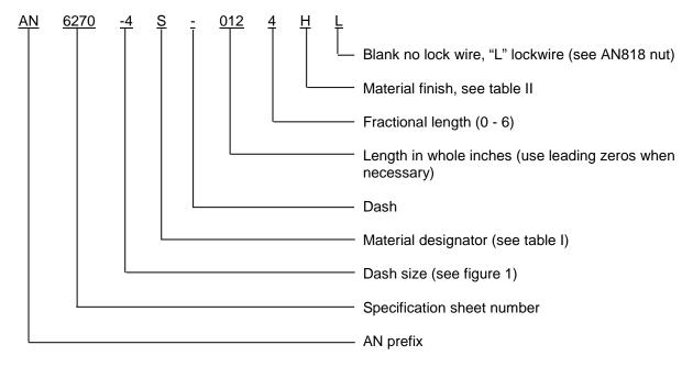
Example of PIN: AN6270-4S-0124HL indicates a hose assembly .250-inch tube to hose, 4140 steel adaptor's, 12.5 inches long, zinc aluminum plating, and lock wire holes.
