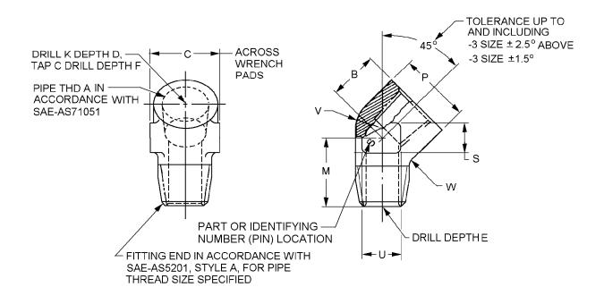
FIGURE 1. Elbow 45° dimensions and configuration.
