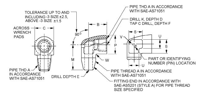
FIGURE 1. Elbow 90° dimensions and configuration.
